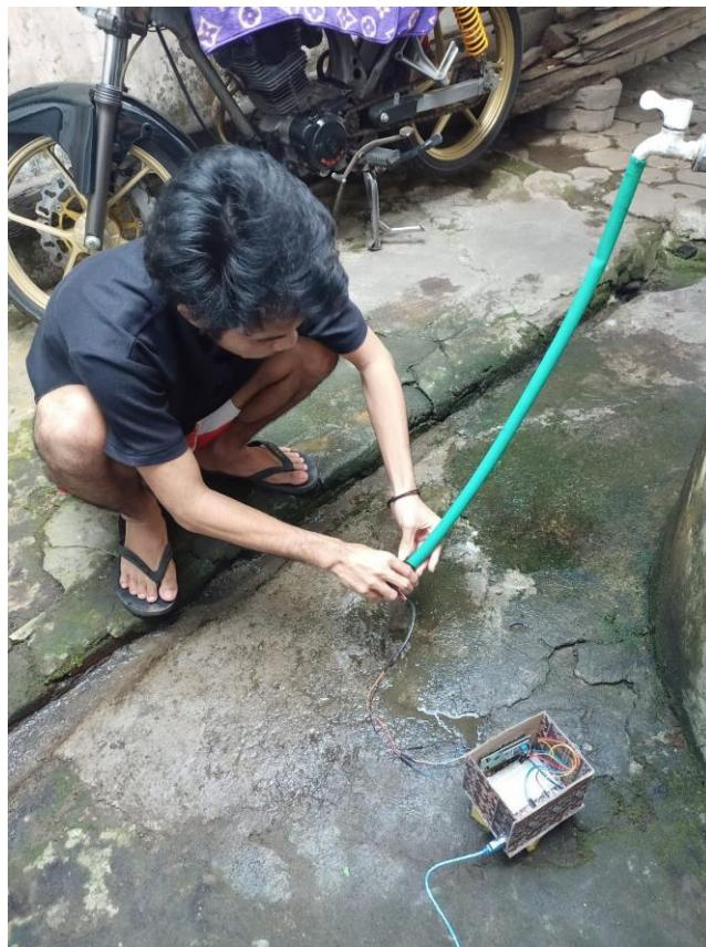
G. Proses Pengujian Sensor Water Flow Dengan Wadah Ukur
