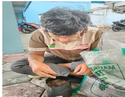
Penguburan sampel biodegradability
