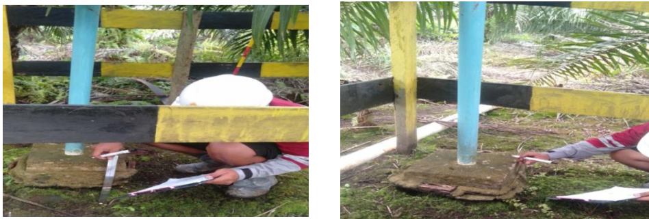
Gambar 4.1. Monitoring Patok subsiden
