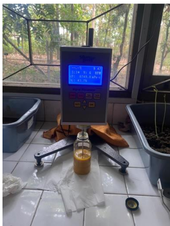
Analisis viskositas Hand and Body Lotion
