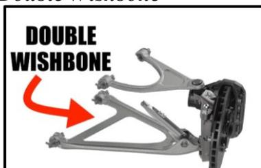
Gambar 27. *Double Wishbone*
