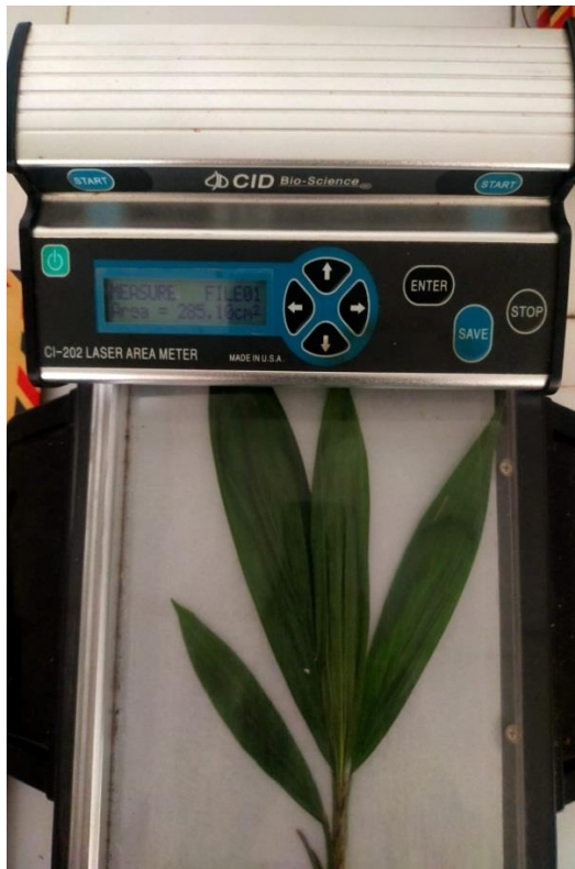
31. Pengukuran daun (leaf area meter)
