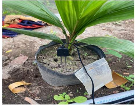
Gambar 4.2 Sensor Kelembapan Tanah Didalam Media Tanam
