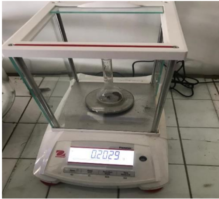
5. Proses Penimbangan sampel tanah
