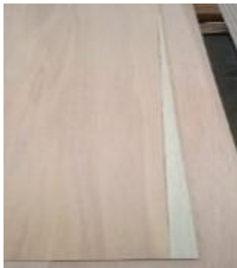
Cacat Teknis Joint Face
