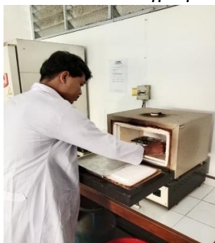
Proses muffle furnace uji kadar abu
